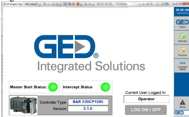
3.2 Intercept i3. To configure the Intercept i3 machine for communication with the Smart Extruder +, a new CPU will need to be installed with the latest plc program. The new CPU has a different IP address so the network settings on the pc will need to be adjusted. The new IP address also needs to be added to the PMAC setup. And then the WinFrame software needs to be configured to run with a Smart Extruder + machine.
