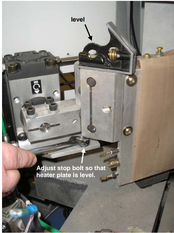
Leveling the Heater Plate
